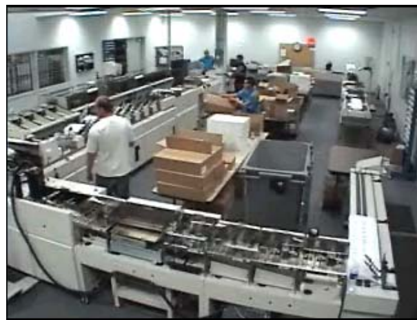
The above image shows the current equipment used to process ballots. We are currently able to process 50,000 mail pieces each day.
