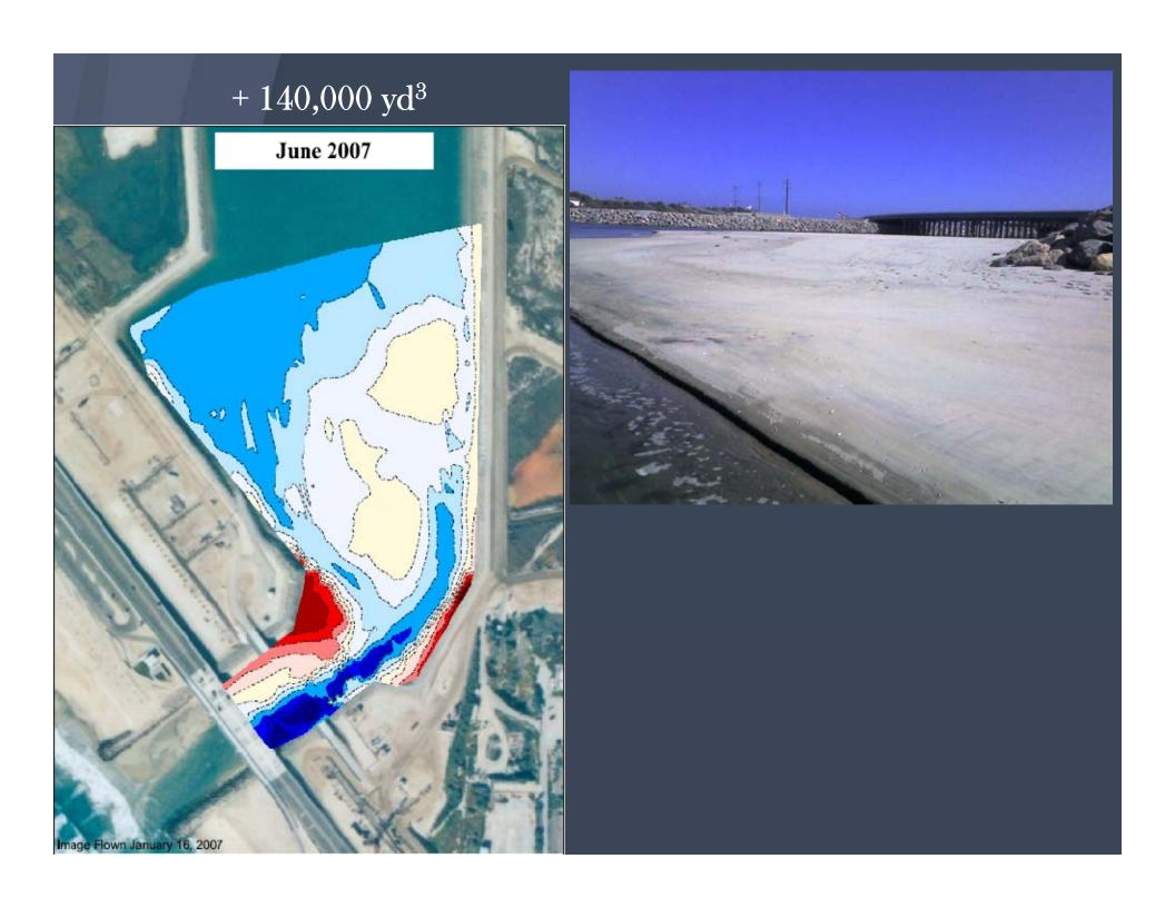
• Monthly Berm & MSL Measurements • Quarterly On/Offshore Profiles New Entrance Channel 2 km
